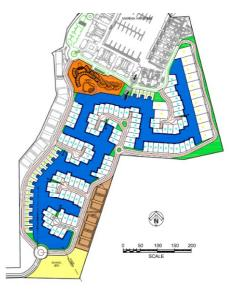
The Inner Harbour has been planned by BPDC to maintain a perched water level within a controlled semi-tidal variation - sufficient to achieve adequate tidal exchange and thereby ensure high water quality, while maintaining an attractively close residential living interface with the water.
